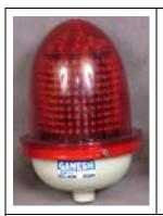
ELECTRICAL DATA ICAO & FAA Norms approved No. Of LEDs: 343 Maximum forward current: 100mA Typical power consumption: 8.8 W Maximum at 230V AC Input voltage variability: Can withstand fluctuation of ±25% PIV protection: LEDs internally protected against rev. voltages up to 1 kV Insulation resistance: >200 megohms at 1000V Dielectric strength: 2.5 kV Earthing: Terminal provided inside body Cable entry: ET 19mm I luminance: @3300 lux
