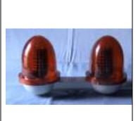
ELECTRICAL DATA ICAO & FAA Norms approved No. Of LEDs: 343 x 2nos./196x2/121x2/50x2/40x2 Maximum forward current: 200mA/140/90/17mA Typical power consumption: 8.8 W x 2 at 230V AC /10w / 7w / 2.5w Input voltage variability: withstand flucn.±25% Insulation resistance: >200 megohms at 1000V Dielectric strength: 2.5 kV Earthing: Terminal provided inside body Cable entry: ET 19mm I luminance: @3300/3300/1700 lux per each lamp
