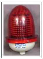
ELECTRICAL DATA ICAO No. Of LEDs: min 175 max 182 nos Maximum forward current: 77mA Typical power consumption: 3.7 W Maximum at 48 V DC Input voltage variability: Can withstand fluctuation of ±15% PIV protection: LEDs internally protected against rev. voltages up to 1 kV Insulation resistance: >200 megohms at 1000V Dielectric strength: 2.5 kV Earthing: Terminal provided inside body Cable entry: ET 19mm I luminance: @30.2 lux at 1 mtr distance
